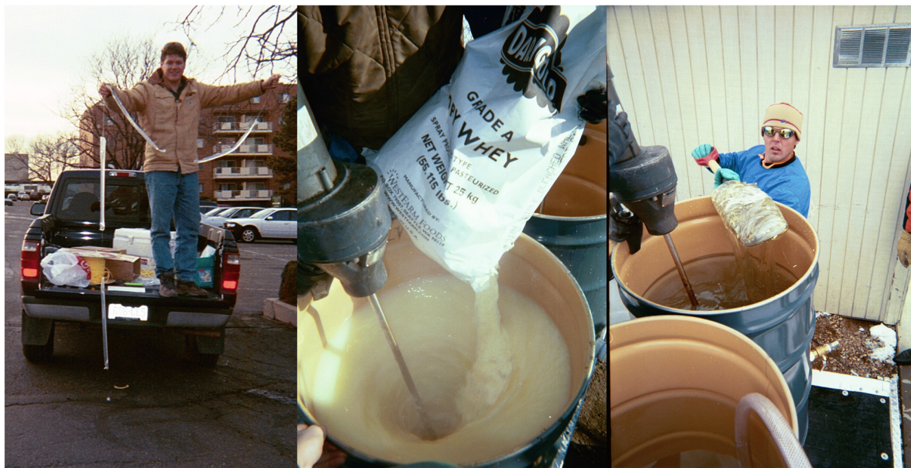
Figure 1. Left: The author during one of the first deployments of commercially available passive diffusion samplers in 2002. The PRP was interested in changing sampling methods because of the cost savings (~25%) offered by the new technology, and therefore was motivated to develop site-specific comparison data to attain regulator acceptance. Center and Right: Preparing whey-based and corn syrup-based reagent solutions prior to injection for an early implementation of ERD in 2001. At this time little was understood about in situ biogeochemical processes, reagent optimization, injection well system design and hydraulics, and the practical effects of heterogeneity and diffusion into and out of low-permeable geologic materials on injected reagent distribution and remediation system performance. This PRP supported this pilot test work because they had a portfolio of chlorinated solvent sites and recognized the large potential benefit of this nascent (at the time) technology.
