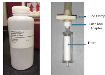
Figure 3: Groundwater samples can be collected in 1 L poly bottles or using Bio-Flo filters
